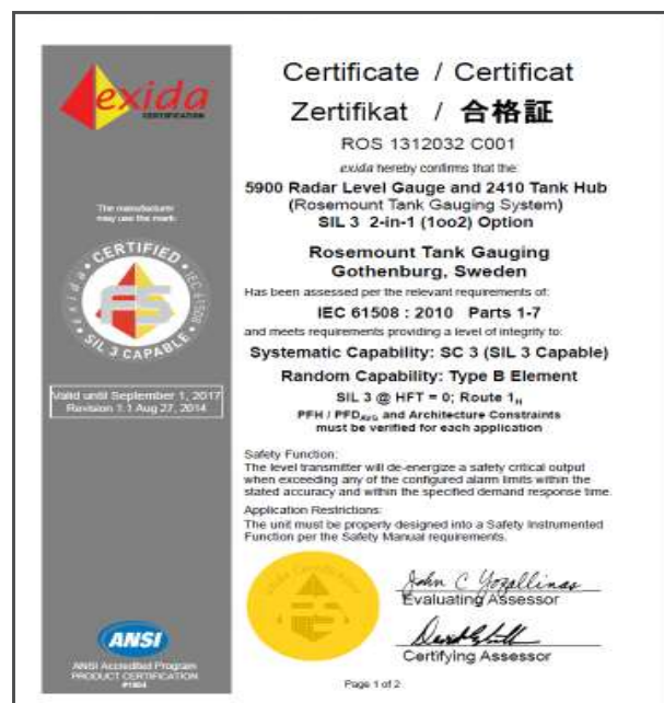
Figure 5.5: Third party assessors generate certificates stating that the equipment conforms to IEC 61508
