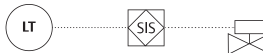
Figure 3.7: Automatic overfill prevention systems (AOPSS) usually consist of a level transmitter (LT), logic and actuator that automatically closes a valve to prevent overfills from occurring. No human intervention is required which usually increases the reliability and shortens the response time
